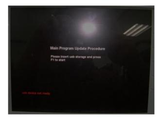
When the <u>xxx.opg</u> or <u>xxx.upg</u> file on USB flash disk has been recognized by oscilloscope, the message "<u>usb device ready</u>" will appear on the lower left corner.
